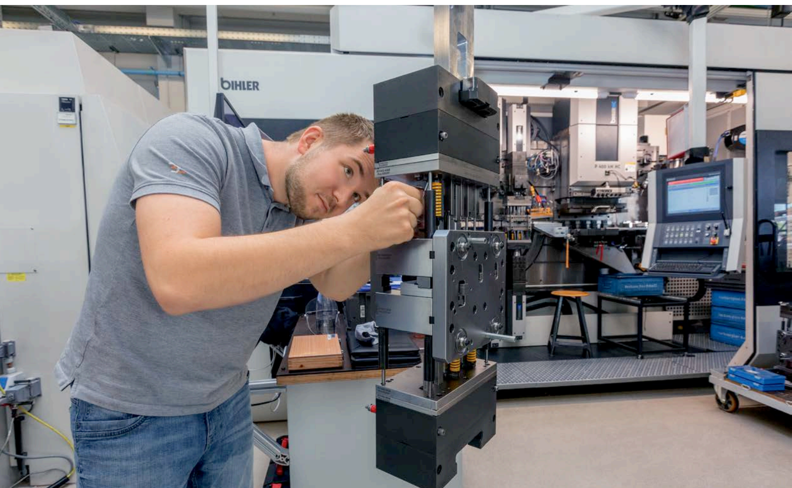
The high-speed clamping component of the Bihler LEANTOOL system ensures short setup times coupled with optimum tool positioning.
