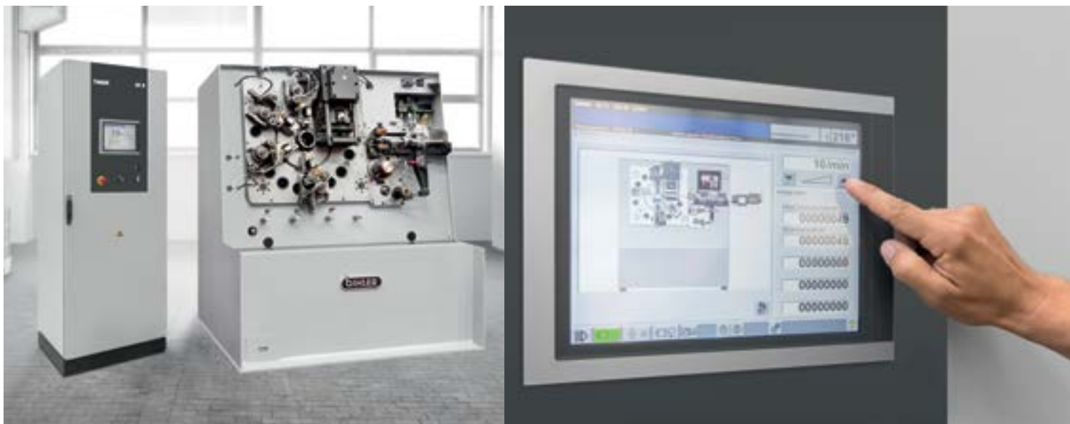
Existing Bihler systems can be modernized within five working days using the BC R upgrade and retrofit package.
