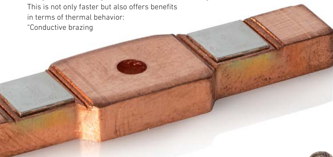
Using the new conductive resistance brazing process, it is possible to apply contacts measuring up to 10 x 10 mm to 5-mm thick copper carrier strips.
