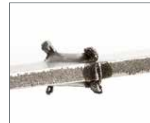
Resistance butt welding
