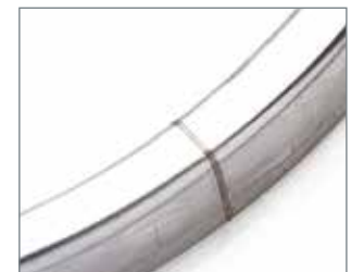
Mash seam welding
